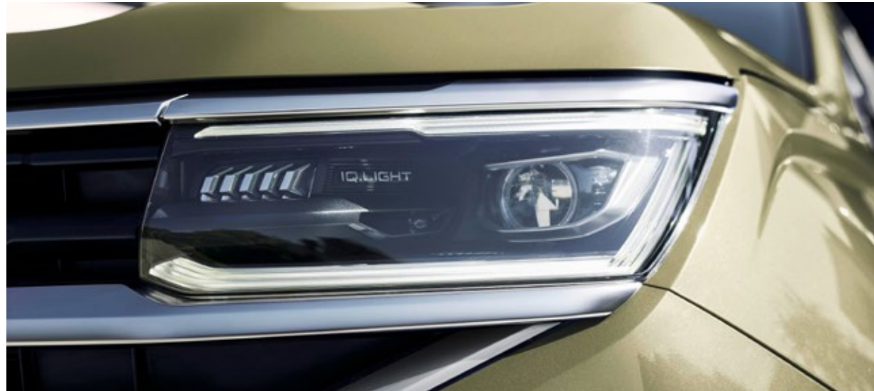
IQ.Light LED matrix headlights standard on Style, Dark Label, PanAmericana, Aventura and W600 models. • With individually activated light emitting diodes to determine the brightness and direction of the light cone, thus providing variable illumination of the road depending on the situation. • Includes the Dynamic Light Assist advanced main beam control and dynamic headlight range control functions.
