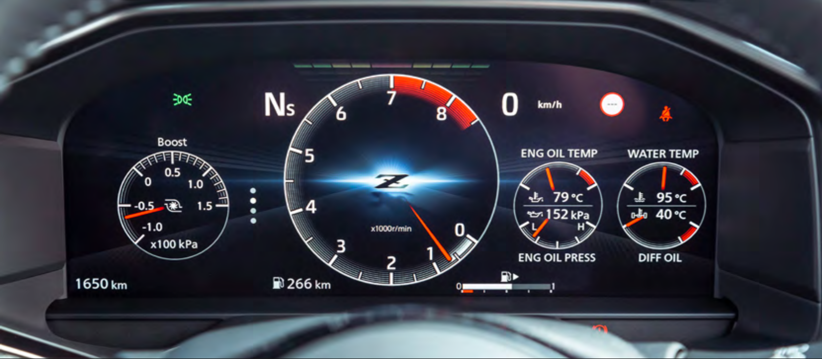
12.3" TFT Advanced Drive-Assist Display instrument cluster
