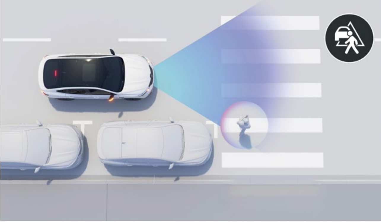
active emergency braking system This detects obstacles such as vehicles, pedestrians or cyclists in front of your vehicle, warns you and will automatically perform emergency braking if you do not.
