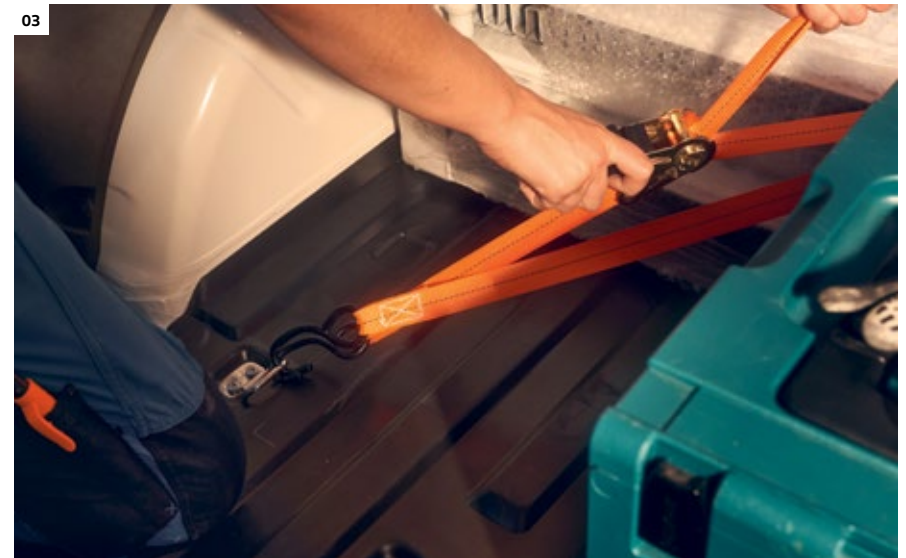
03 Lashing eyes. Keep their promise. The six folding lashing eyes secure heavy loads rock-solid on the vehicle floor of the Caddy Cargo. | C |
