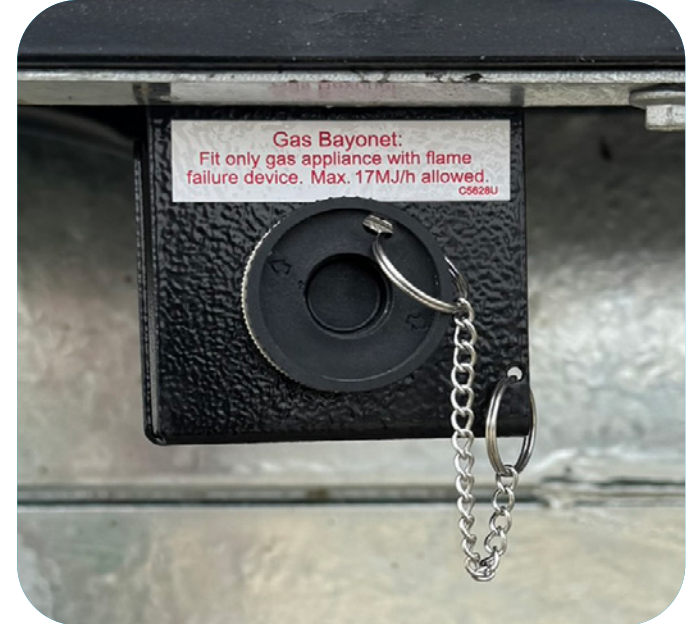
Side mount under chassis gas bayonet for easy access to gas for external cooking
