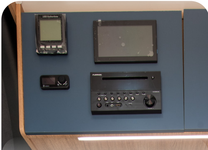
Modern tech upgrades include the new 7" Projecta control panel and Furrion stereo with external speakers
