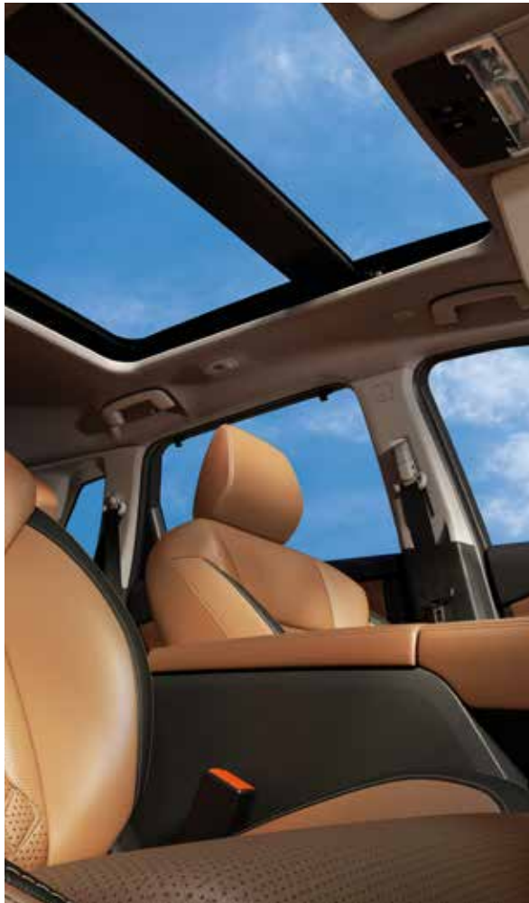
Tilt & slide power sunroof with panoramic glass roof*
