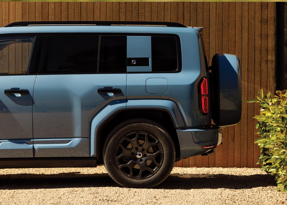
With a 3-tonne towing capacity and up to 600kg payload, there isn't much the DENZA B5 can't move. A drawbar, hitch receiver and 12 pin plug are all included as standard fitment. The DENZA B5 LEOPARD fitted DiSus-P will even self level if it detects any sagging.
