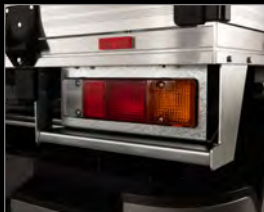
Tail Light Protector & Wiring Guard
