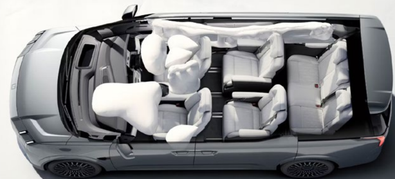
7-airbag system covers all three rows
