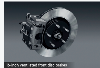
16-inch ventilated front disc brakes
