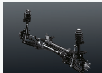
16-inch Monroe® MacPherson strut on the front suspension
