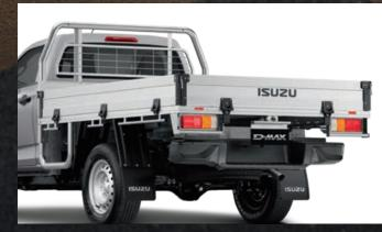
**Heavy Duty Alloy Tray**<sup>#</sup> - All features of the General Purpose Alloy Tray with a tube headboard and integrated tray step (on single cab trays only).
