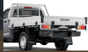
**General Purpose Alloy Tray**<sup>#</sup> - Standard alloy tray with added welded wire mesh window protector and tail light protectors.
