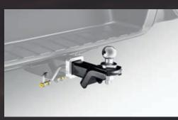
**Tow Tongue Kit** (Cab Chassis long & Ute tub short kits are available; compatible with LS-U range & X-TERRAIN)
