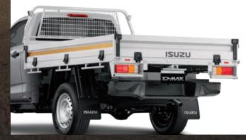
**Mine Specification Steel Tray**<sup>#</sup> - A sturdy steel tray with reflective side striping, a steel mesh window protector and headboard aerial mounts. Available in Mineral White only.
