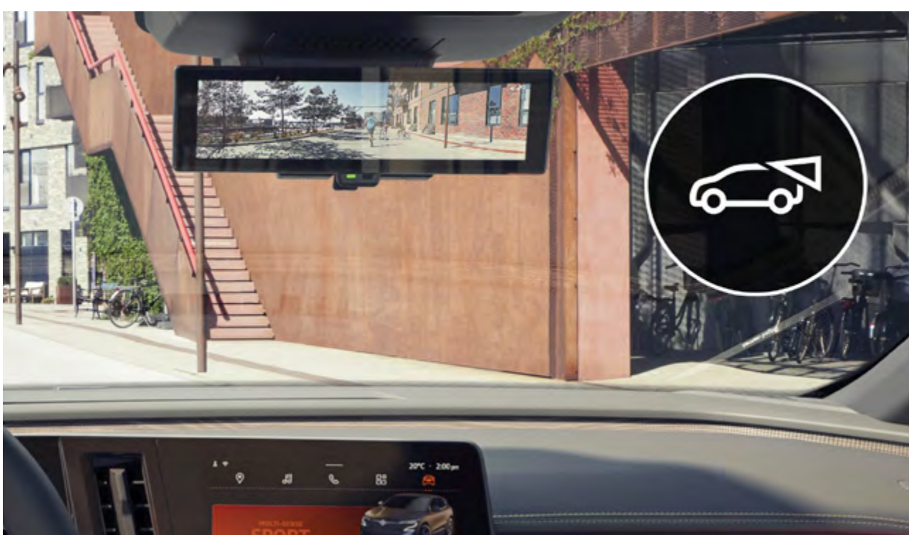
smart rear-view mirror This system uses a camera fitted at the top of the vehicle's rear window, with the interior rear-view mirror showing the clear, unobstructed view image of the road from the rear.
